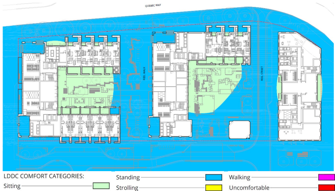
Figure 23 (above): Expected wind conditions at ground level in the windiest season pre-mitigation, modelled on a context comprising the proposed development plus the entire CWM and cumulative surrounding buildings.
