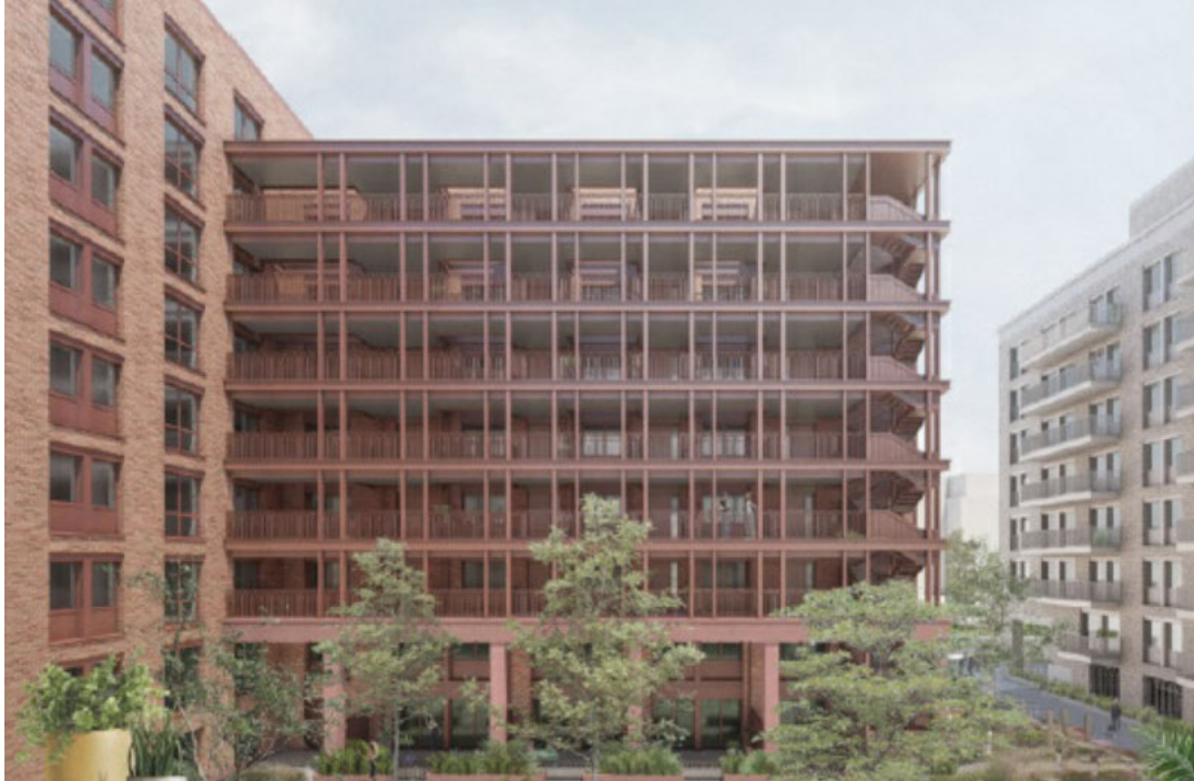
Figure 45 (above): Visualisation of the southwestern side of Block L1's Quebec Way wing, showing the deck access arrangement from second floor upwards.
