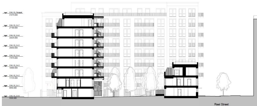
Figure 38 (above): Northeast-to-southwest section through Block L1, showing the eight storey wing fronting Quebec Way the three-storey wing fronting Reel Street with the courtyard in-between. In the background, Block L2 can be seen.
