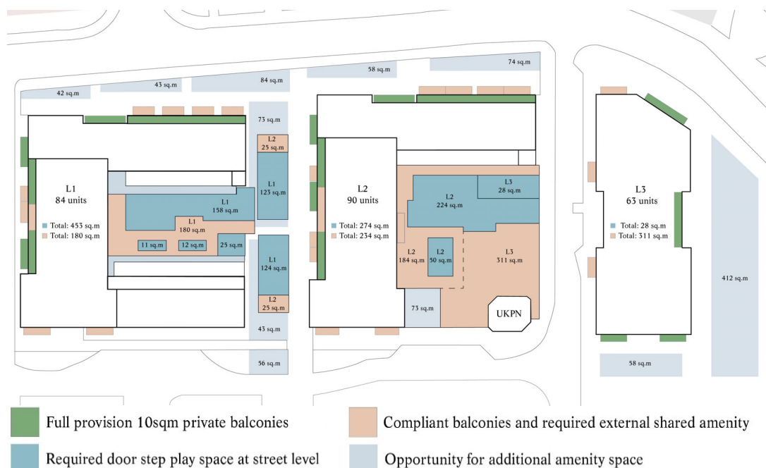
Figure 28 (above): Schematic of play, communal amenity and additional public amenity space across Zone L, including the northern section of Park Walk.
