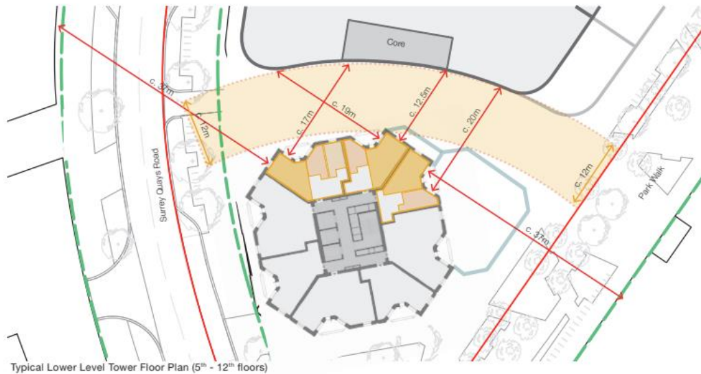
Image: Plan typical separation distances between F1 and F2 (5 th -12 th floors)
