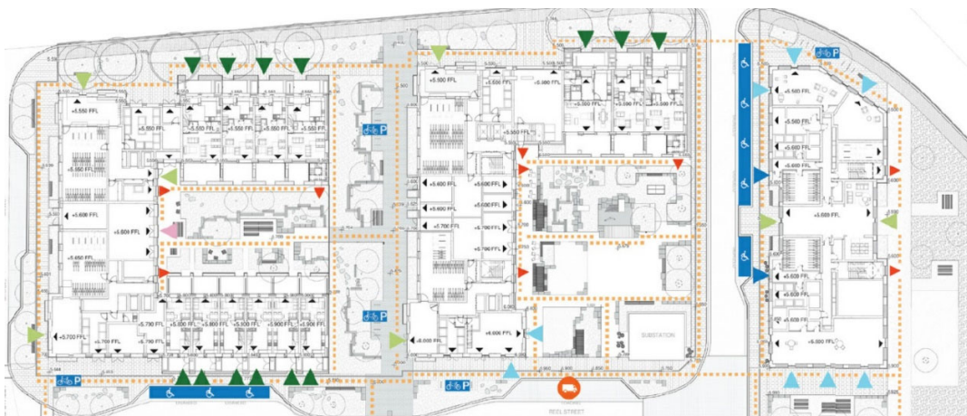
Figure 61 (above): Ground plan of Zone L, with the Blue Badge bays shown in dark blue. Entrances to the residential lobbies are denoted by light green triangular arrows.
